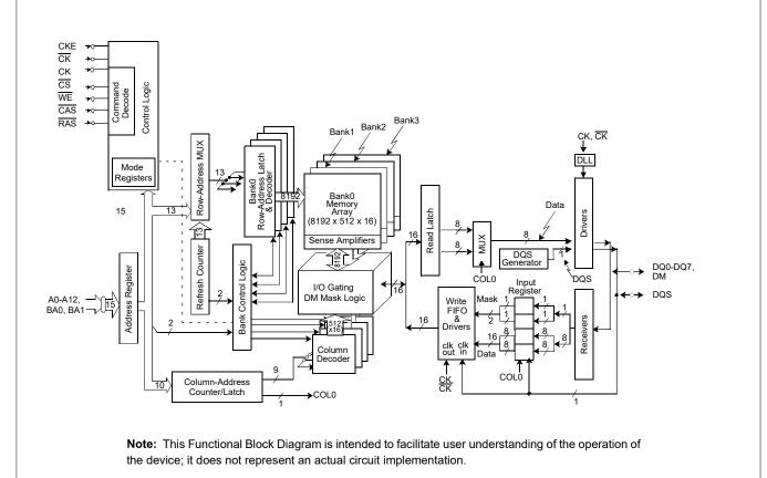
**Note:** DM is a unidirectional signal (input only), but is internally loaded to match the load of the bidirectional DQ and DQS signals.
