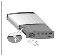
4. Use a screw driver to secure the case and stand with the two remaining screws.
