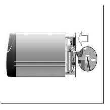
3. Push the hard disk and plastic base back into the case, careful to align the plastic base to the aluminum housing.
