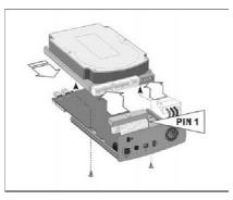
2. Plug the cable of the LED into the connector on the PCB.
