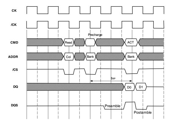
Figure 6. Precharge Termination of a Burst Write (Burst Length=4)
