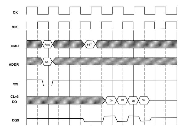
Figure 10. Read Terminated by Read (Burst Length=4, CAS Latency=3)
