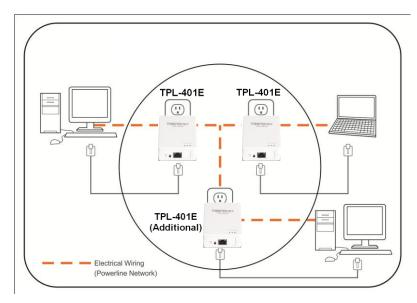
Assuming the two TPL-401E powerline adapters are currently connected to each other and the third TPL-401E (Additional) powerline adapter is currently disconnected.
