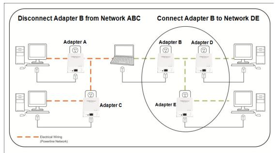
Assuming all powerline adapters are TPL-401E adapters and for reference in the diagram and this procedure, the adapters will be labeled *Adapter A, B, C, D,* and *E. Adapters A, B,* and *C* are currently connect together to form one powerline network and *Adapters D* and *E* form another powerline network. *Adapter B* will be disconnected from *Adapters A* and *C* and connected to *Adapters D* and *E*.
