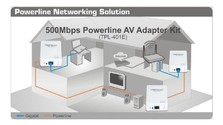
The example diagram shows a typical powerline network configuration in a home environment with 3 powerline adapters installed in different rooms. The orange line represents the powerline connectivity established through your home's electrical system and the blue lines represent Cat. 5, 5e, 6 Ethernet connectivity to your network enabled appliances such as a computer, router, or IP set top box connected to your television.
