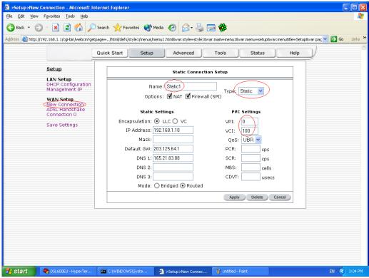
Figure 8 (Static IP Connection Setup)
