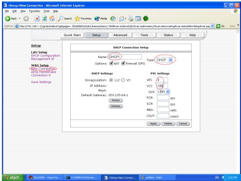
Figure 7 (DHCP Connection Setup)
