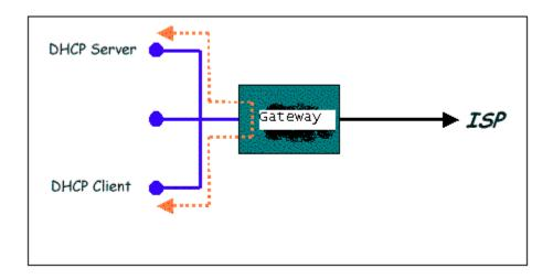
Figure 11 (Example of a DHCP Relay configuration)
